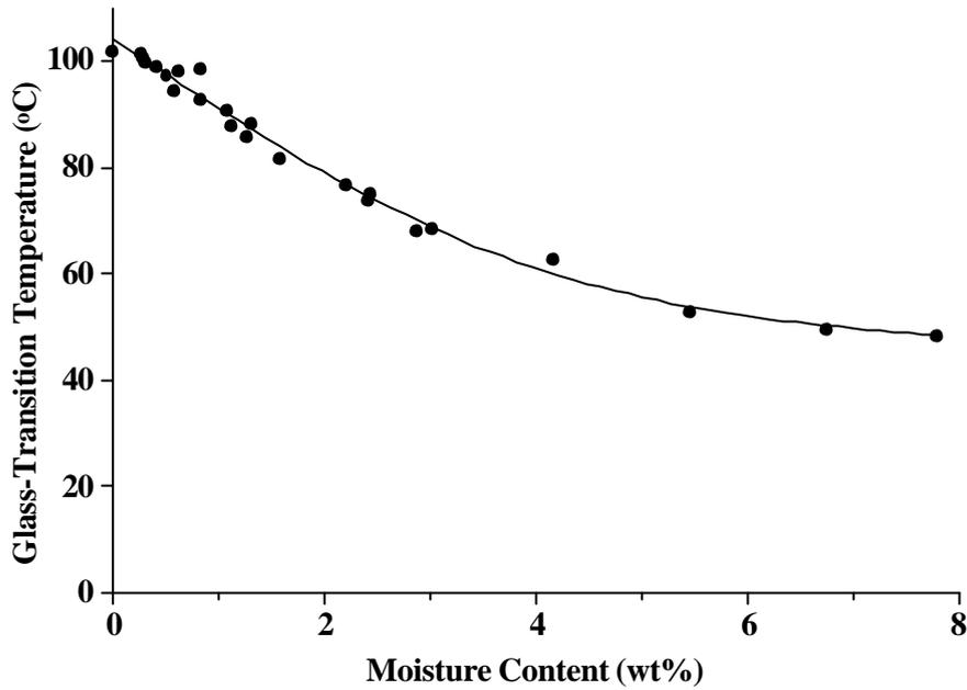
Figure 8 Glass-transition temperature of AV119 as a function of moisture content [2].
