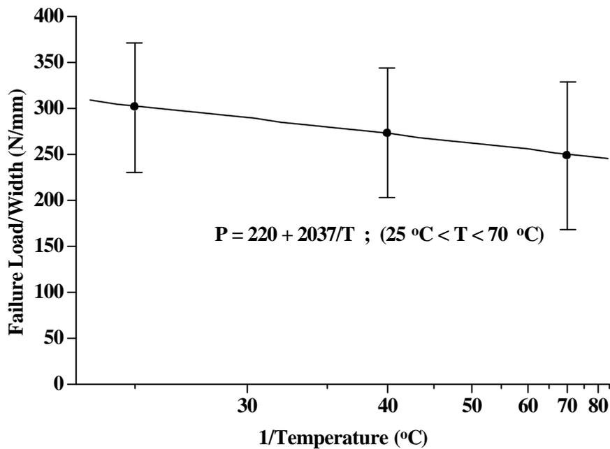
Figure 13 Effect of temperature on failure load for 6Al-4V-Ti alloy/AF126 single-lap joints.
