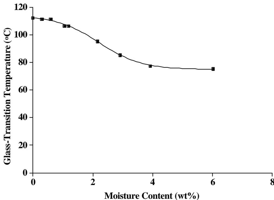
Figure 17 Glass-transition temperature of AF126-2 as a function of moisture content.
