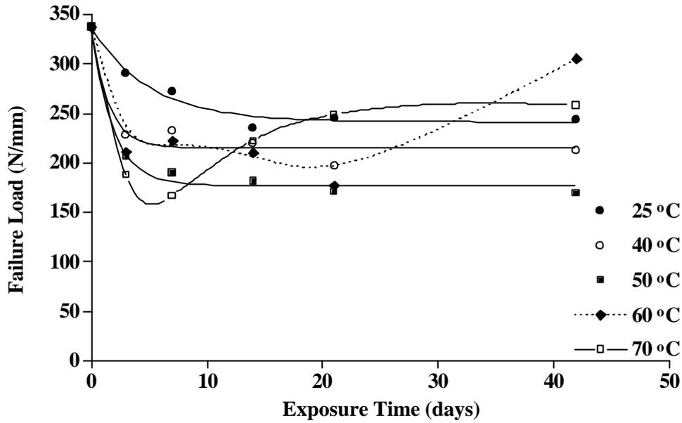
Figure 5 Strength retention of moisture conditioned CR1/AV119 single-lap joints.
