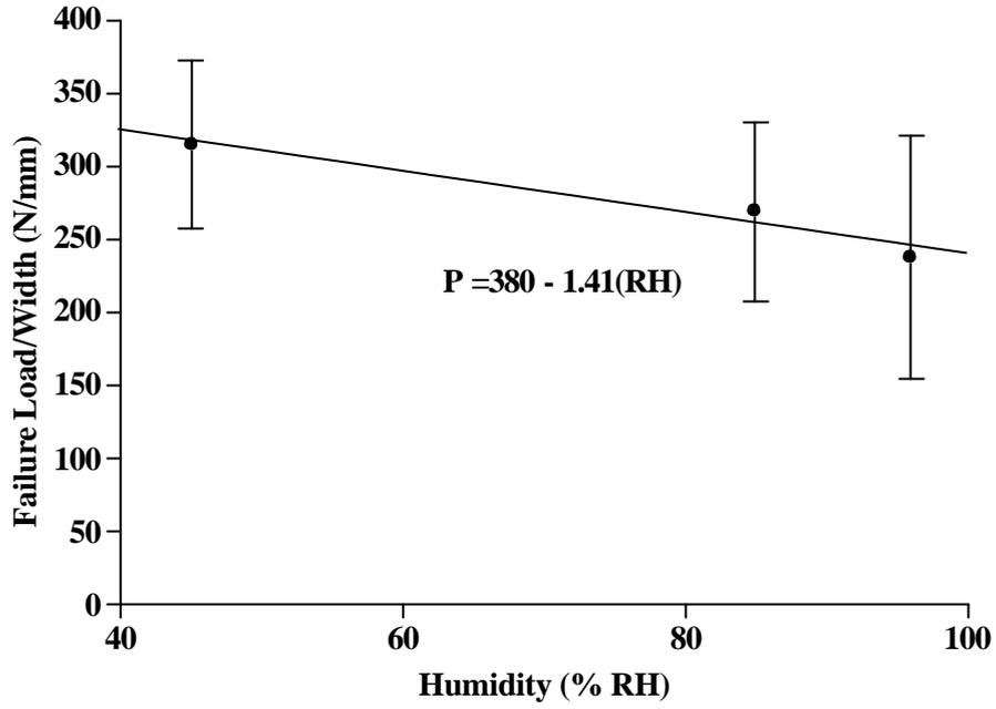
Figure 14 Effect of humidity on failure load for 6Al-4V-Ti alloy/AF126 single-lap joints.
