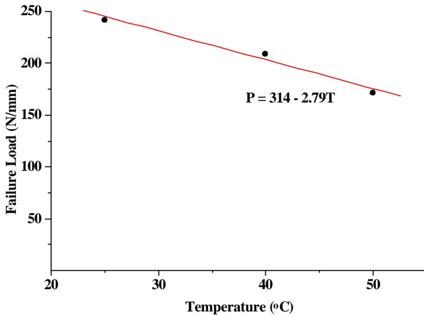
Figure 7 Strength limits for CR1/AV119 single-lap joints.
