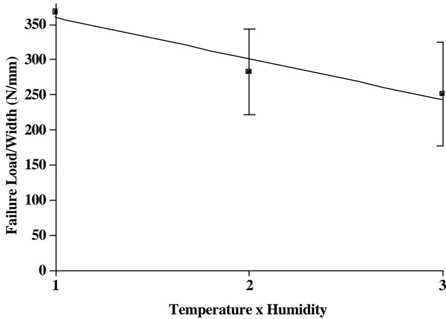
Figure 16 Interaction between temperature and humidity.
