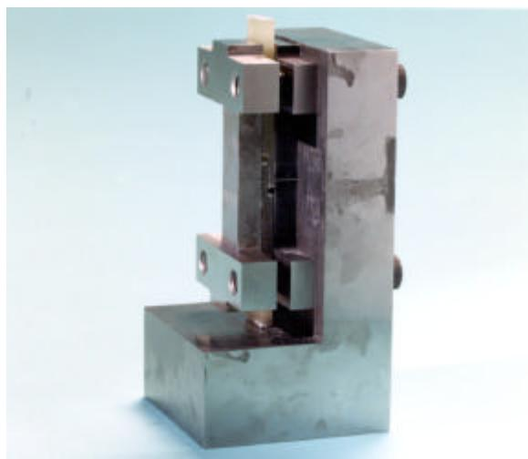
Figure 3 Compression fixture with TAST specimen.
