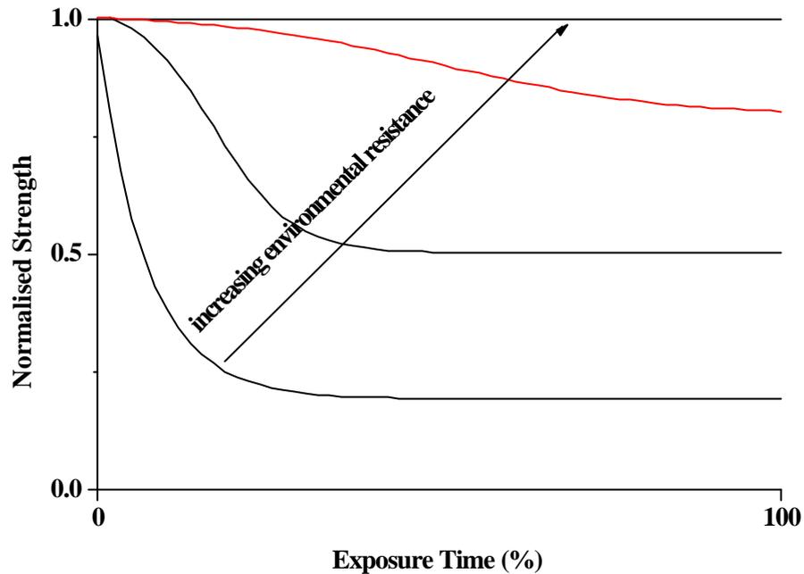
Figure 18 Schematic of typical strength reduction with exposure time curves.
