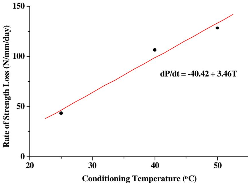
Figure 6 Rate of strength loss over first 3 days exposure for CR1/AV119 single-lap joints.
