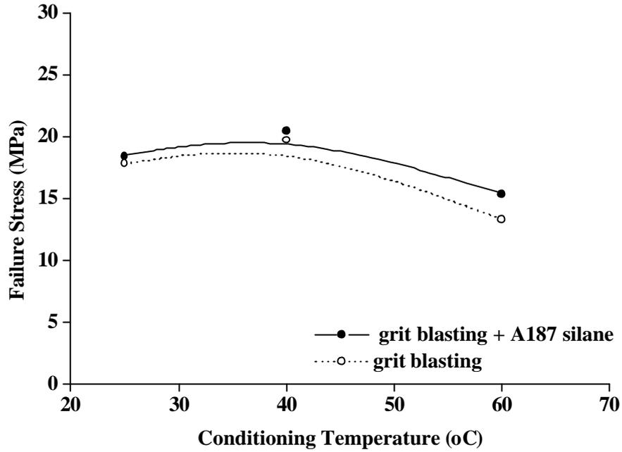
Figure 11 Failure stress after 42 days water immersion for F241 TAST specimens
