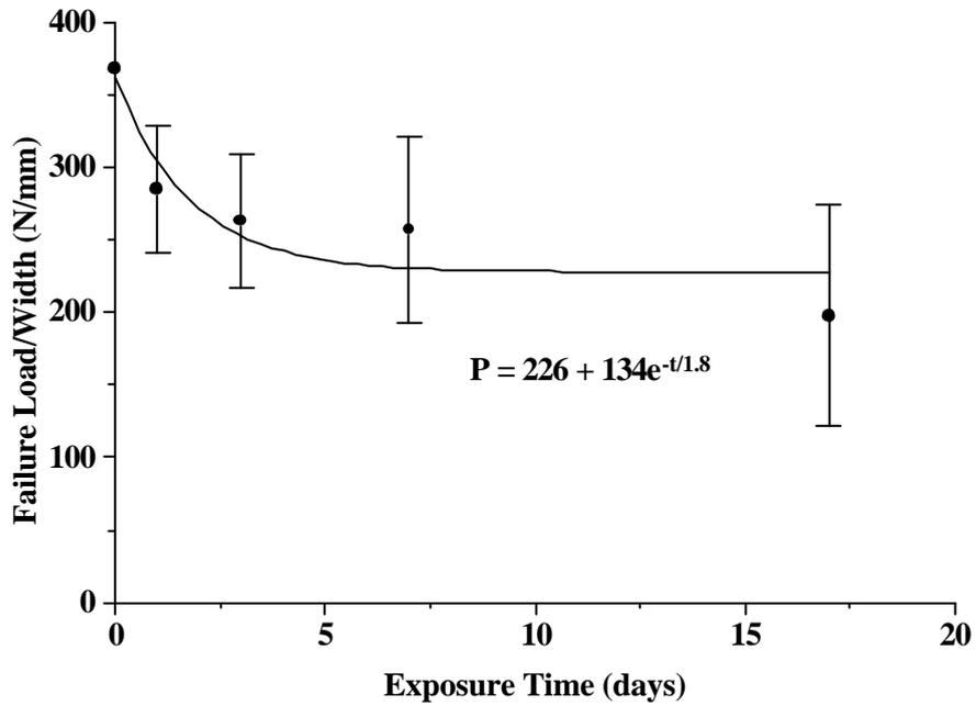
Figure 15 Effect of time on failure load for 6Al-4V-Ti alloy/AF126 single-lap joints.
