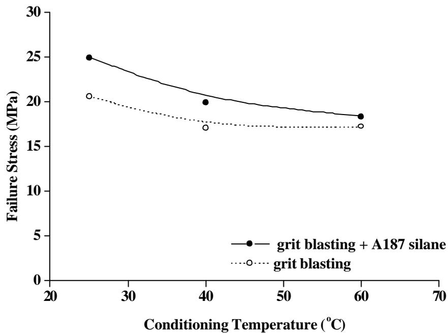
Figure 10 Failure stress after 42 days water immersion for AV119 TAST specimens
