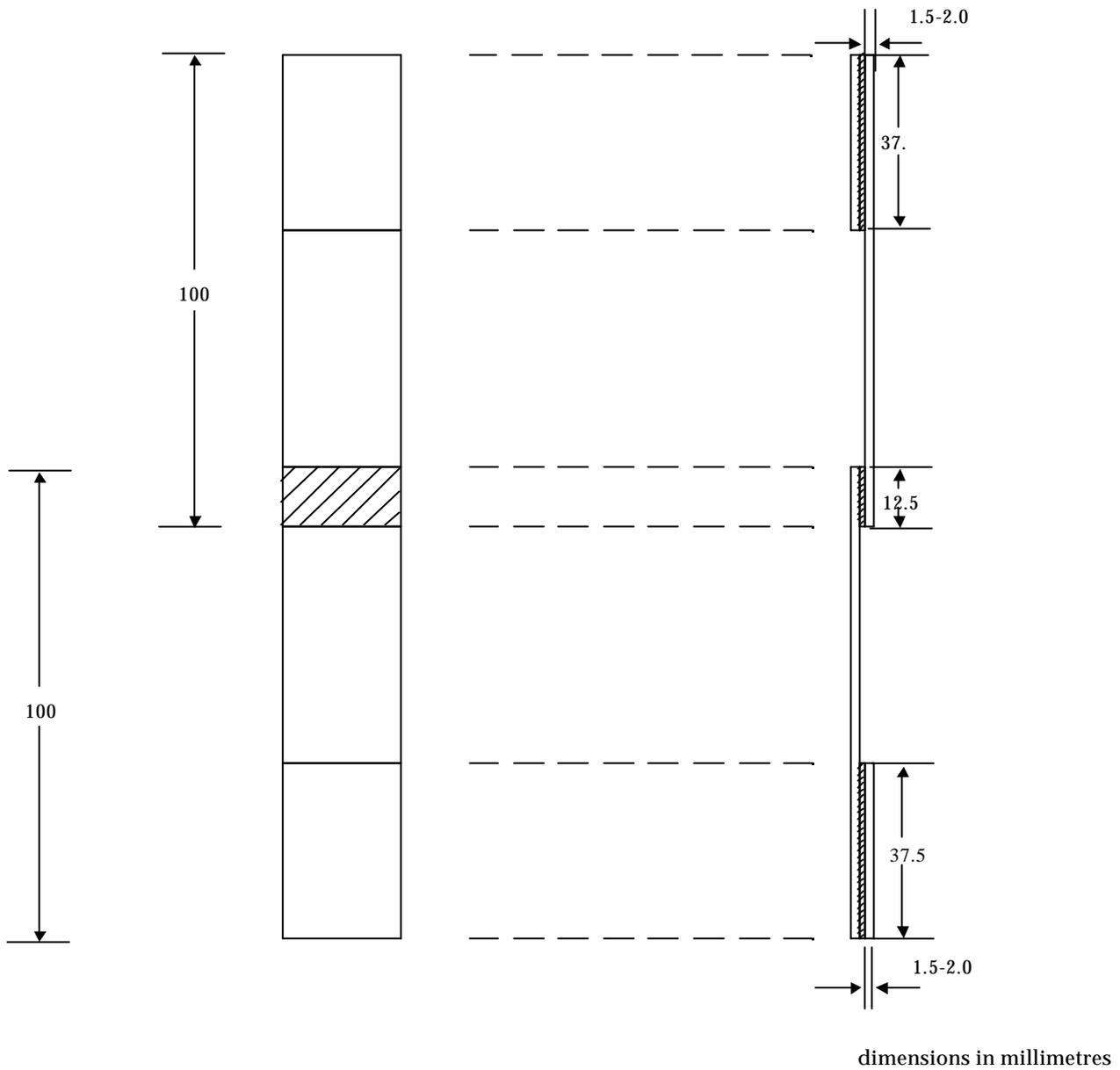
Figure 4 Schematic of single-lap joint.
