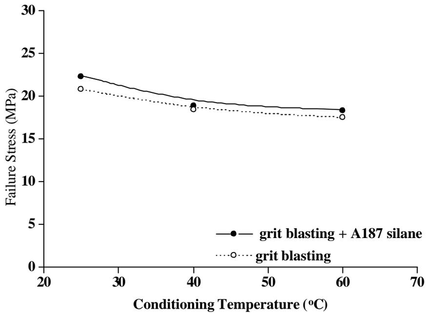
Figure 12 Failure stress after 42 days water immersion for AF126-2 TAST specimens.
