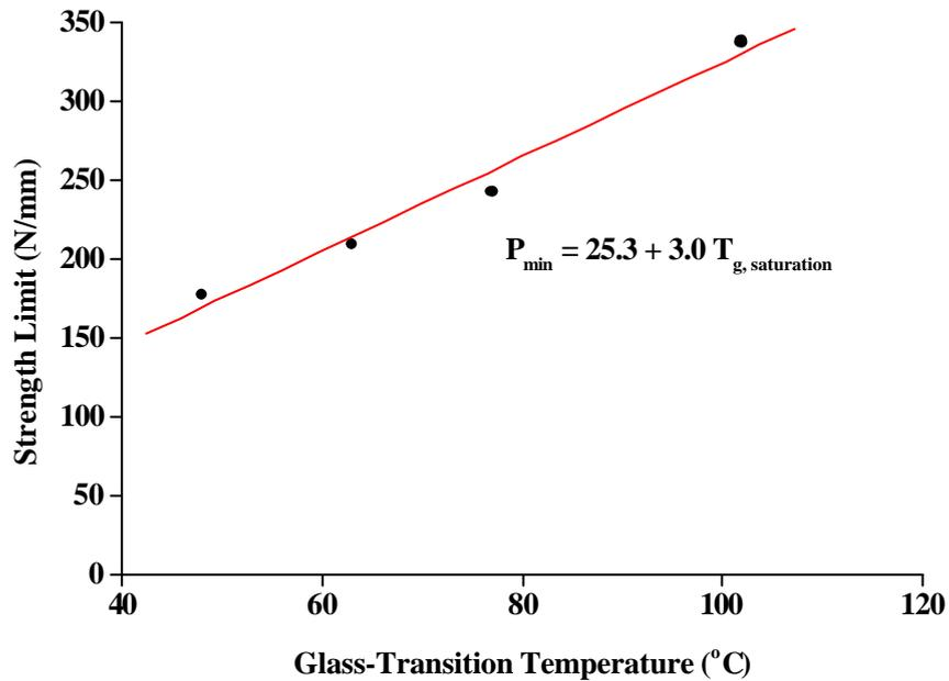
Figure 9 Minimum joint strength versus the saturation value of **T<sub>g</sub>** for AV119 bulk resin.
